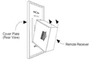
Position the receiver as shown in diagram to the left with lower tab on cover plate inserted into groove of receiver (Make sure ADJ hole and LEARN hole on cover plate properly aligns with remote receiver) Pull Receiver up and snap into top tab of cover plate.
