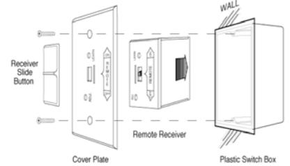
NOTE: The remote receiver will only respond to the transmitter when the 3-position slide button on the remote receiver is in the REMOTE position. If the system does not respond to the battery transmitter on initial use, see MATCHING SECURITY CODES, and recheck battery positions in the remote receiver.
