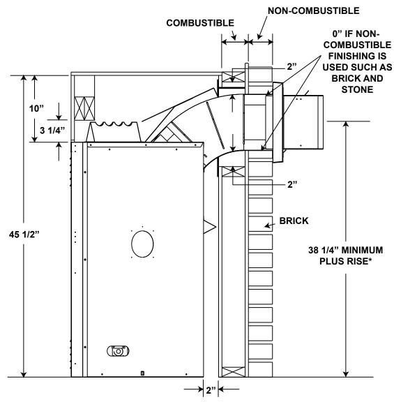
The appliance requires a minimum enclosure height of 45 1/2". For temperature requirements, the enclosure space around and above the appliance must be left unobstructed.
