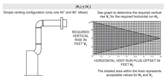
For vent configurations requiring more than one 45° elbow and 90° elbow, the following formulas apply: Formula 1:  $H_{\tau} \leq V_{\tau}$ Formula 2:  $H_{\tau} + V_{\tau} \leq 40$  feet
