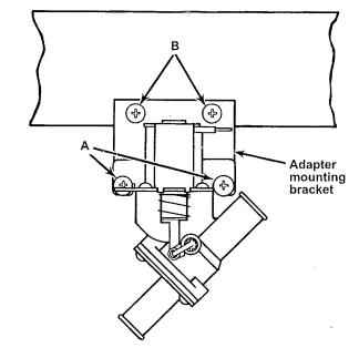
The special adapter mounting bracket included in the kit must be used to properly locate the drain valve on the dishwasher cross channel.
