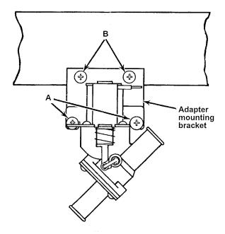
The special adapter mounting bracket included in the kit must be used to properly locate the drain valve on the dishwasher cross channel.
