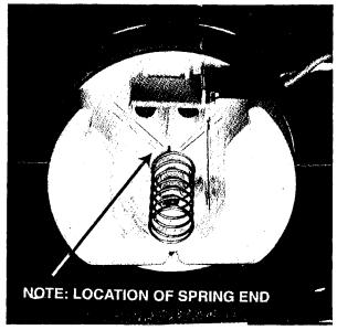
Place cam over spring and shaft for detergent cup cover, making sure end of spring is aligned into window of "V"stop on cam.
