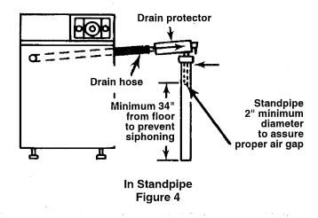
**NOTE:** The drain protector will require periodic cleaning. Unlatch the cover and remove the element for cleaning. Make sure the cover is tightly closed and latched after cleaning.
