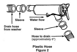
**NOTE:** We recommend using a short piece of drain hose (approximately 6") on the outlet end of the drain protector.
